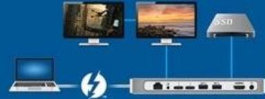
Now, one compact port provides Thunderbolt 3 data transfer, support for two 4K 60 Hz displays, and quick notebook charging with a single cable.
